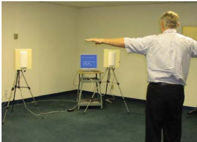
▲ Fig. 5 A typical setup using two units in a bistatic configuration.
