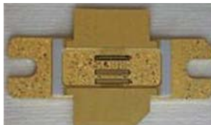
▲ Fig. 1 Top view of the unlidded CPC package with a device A and its input matching network.
