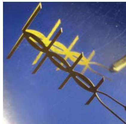
▲ Fig. 4 A 0.010" brass antenna fabricated using Quick Circuit.
