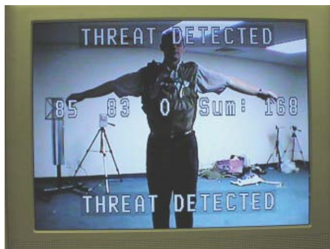
▲ Fig. 3 Output screen showing the information presented to an operator.
