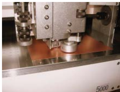
▲ Fig. 2 A 0.016 mil thick microwave substrate being milled on a cushion of air as it is held in place by the Pneumatic Pressure Foot.
