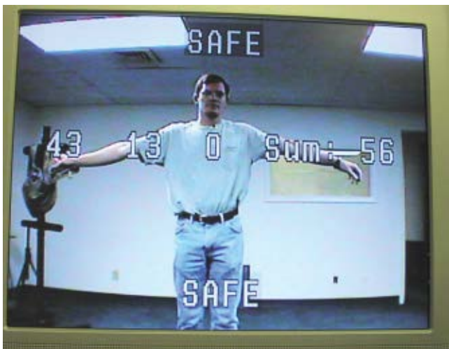
▲ Fig. 6 Output screen showing a SAFE decision along with the person's score superimposed on a visual image of the person being screened.
